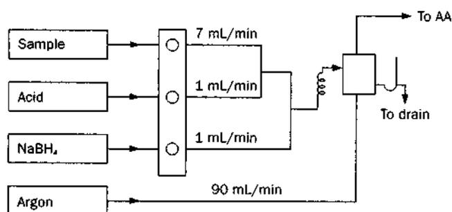
Figure 3114.2. Schematic of a continuous hydride generator.
